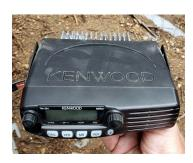
We just got a Kenwood TM-281 from a Silent Key's family. It is 65 Watts and has the magnetic mount antenna. No mounting bracket.
